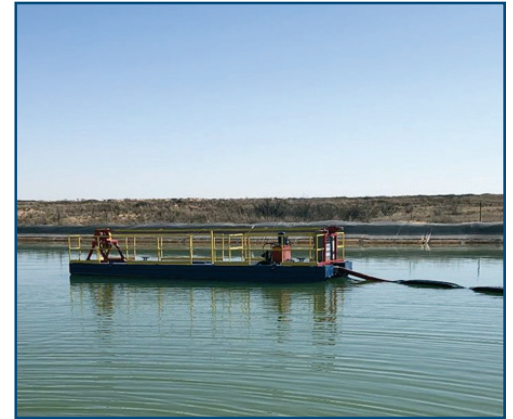
A Mud Cat 40E 30 ft. DD dredge cleans out an aggregate wash plant pont in Texas.
